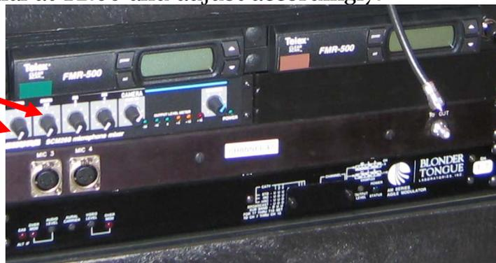
3. If you are going to use the wired microphone, you must first plug one end of a microphone cable into the microphone and the other end into the cart in to either MIC 2 or MIC 3. The volume can then be adjusted using the controls labeled MIC 3 or MIC 4. If you have the microphone plugged into MIC 3 then you will need to adjust the volume for MIC 3. Start the Dial at 12:00 and adjust accordingly.
